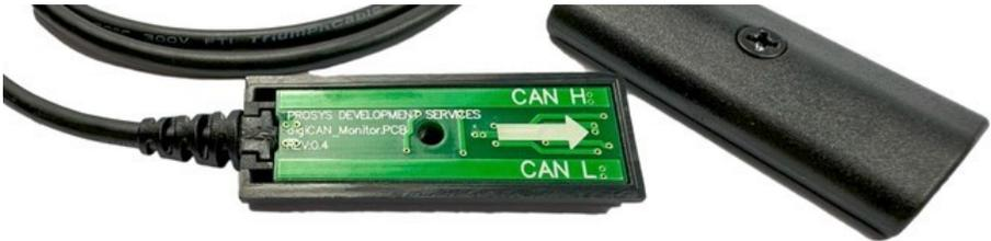
The digiCAN-Slide places the wires over the sensors as you slide the case cover back on. If you are temporarily monitoring you don't need to replace the Philips screw.
