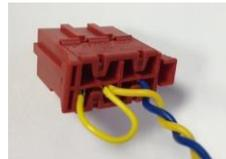
**C-CAN wiring including CAN termination**
